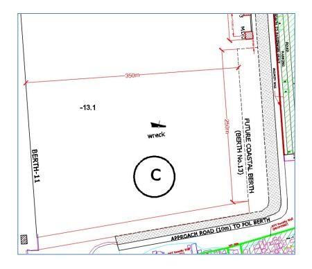
It is proposed to construct a Berth for the promotion of Coastal Cargo in line with 'Development of Berth for Liquid bulk (Petroleum products including LPG)' and Multipurpose General cargo perpendicular to the existing Berth No. 11 to cater to general cargo. Coastal Cargo Berth will be of length 250m opposite to the Berth No. 11 at a distance of 350m away and Multipurpose General Cargo Berth will be of length 350m.
