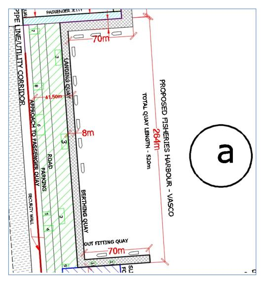
Fishing activities within Vasco Bay is one of the major limitations for expansion of the Port. It is therefore, proposed to construct fishing jetty along with allied facilities. Existing facility is a temporary fish landing platform which is inadequate considering the number of trawlers operating from Vasco Bay.
